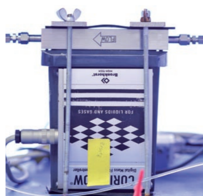
Mass flow controller, a prerequisite for well defined mixtures
