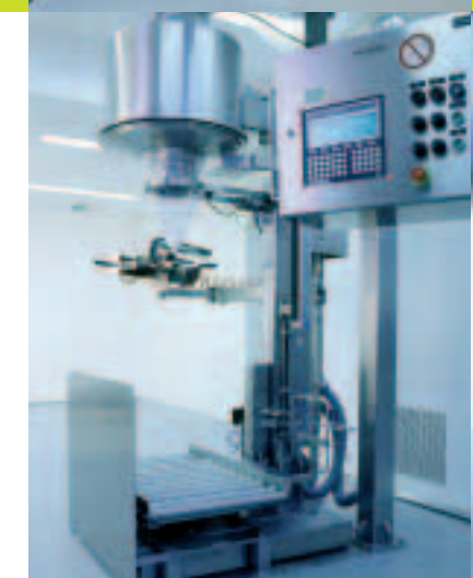
Packaging unit with automatic weight control and continuous bag system
