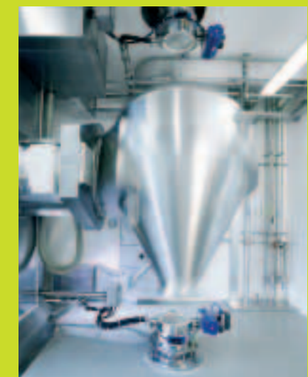
Blender in rotation between «split butterfly valves» (Buck®-type)
