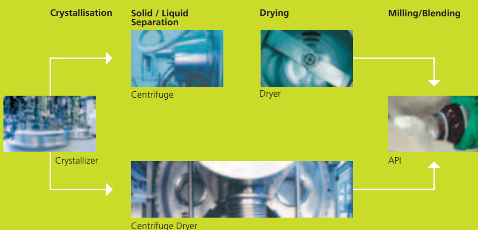
Fig. 1 Final steps of API manufacturing
