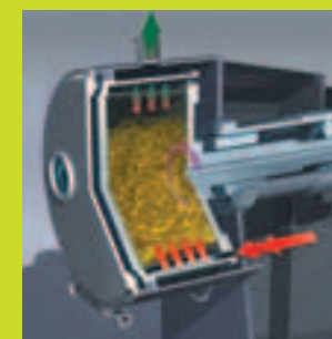
Fig. 3 Fluidized bed drying
